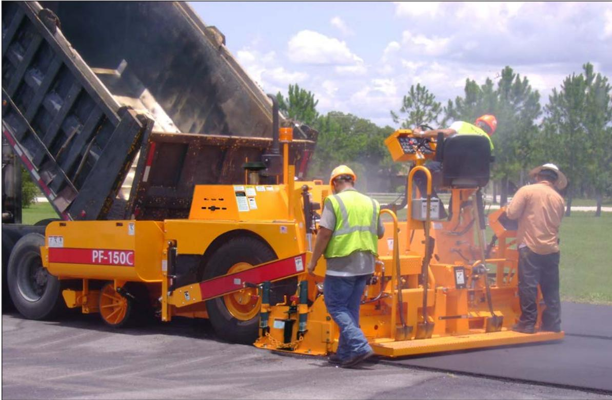
The PF-150C is a heavy-duty, wheel-mounted, paver/finisher, capable of placing bituminous base, binder and surface course mixes, w cement or lime-stabilized sub-base and graded aggregate materials.
