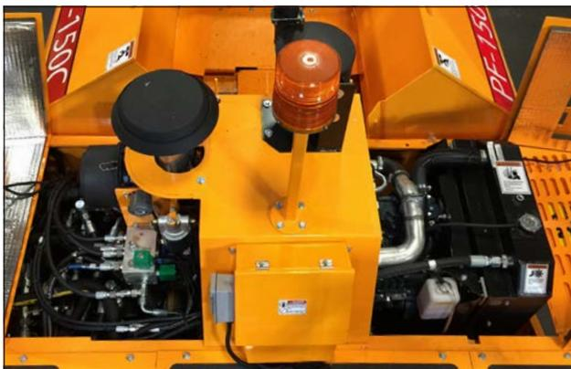
**Cooling System:** Multi-wing fan, pitch configured for optimized systems cooling. Capacity is 4 gallons (15.3 L).
