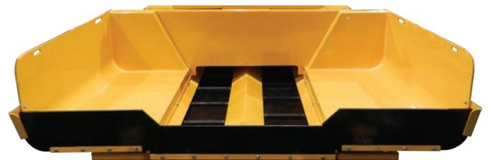
**Dual Feed Systems:** Separate hydrostatic drive for left and right side feed systems provide optimum auger-conveyor operation through the machine's entire capability range. Left and right proportional systems function independently and operation is controlled either manually with electrical switches on the operator's console or automatically by sonic sensing systems positioned at the outer end of each screed extension.
